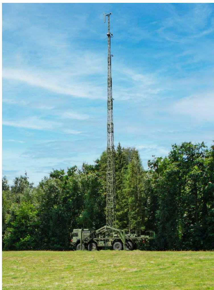
Fth 40/9 – Guyless antenna mast, height 40 m
